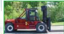
TAYLOR T520M MAST 11' FT, 52,000 LB CAP, 96" FORKS, DIESEL, PNEU TIRES, PS TRANS, CAB W/AIR, SS, FP.
